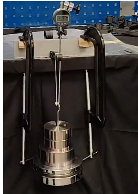
Figure 4: Add metal weights and measure results with a dial indicator
