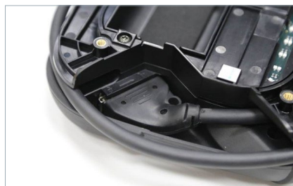
The double-cranked connector geometry is where the challenge arises with the connection cable for the diagnostic device.
