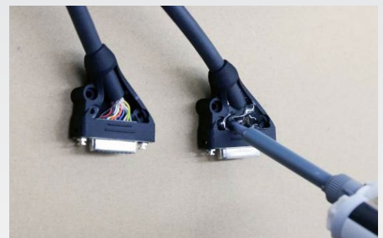
During the final assembly, the pre-assembled plug-cable combination is inserted into the lower part of the housing, encapsulated with a 2K mass and then sealed.
