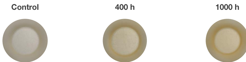
Effect of UV exposure on color of the specimens
